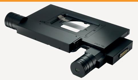
The H101A has an adaptation system to allow one universal stage to fit many microscopes. The stage is compatible with sample holders for up to four standard slides, semiconductor wafers, metallurgical specimens, Microtitre plates or Petri dishes. Incorporating the Prior IST system, this stage is reliable, versatile and precise and is controlled via Prior's versatile ProScan® system.
